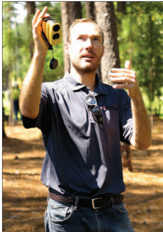
Kelly Bellar, of Laser Technology Inc. ( lasertech.com ), demonstrates the use of the company's TruPulse 360/B laser rangefinder/hypsometer. Horizontals
