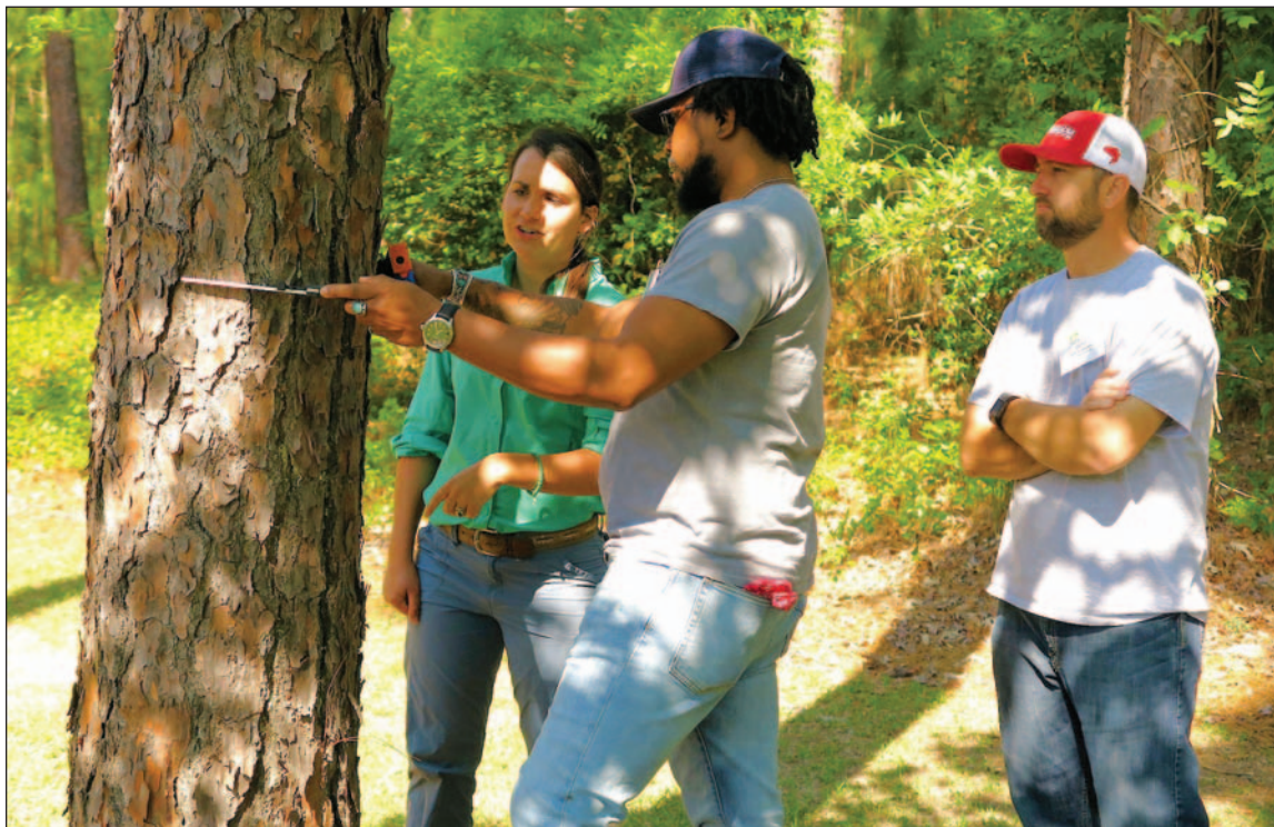
Britt Townsend, of Landmark Spatial Solutions ( landmarkspatialsolutions.com ), explains how to use Haglof MD II electronic calipers
