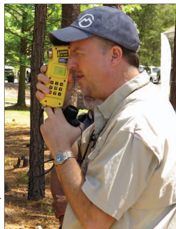
Darian Yawn, of Landmark Spatial Solutions ( landmarkspatialsolutions.com ), demonstrates Laser Technology's Criterion RD 1000 electronic basal area factor scope and densiometer.
